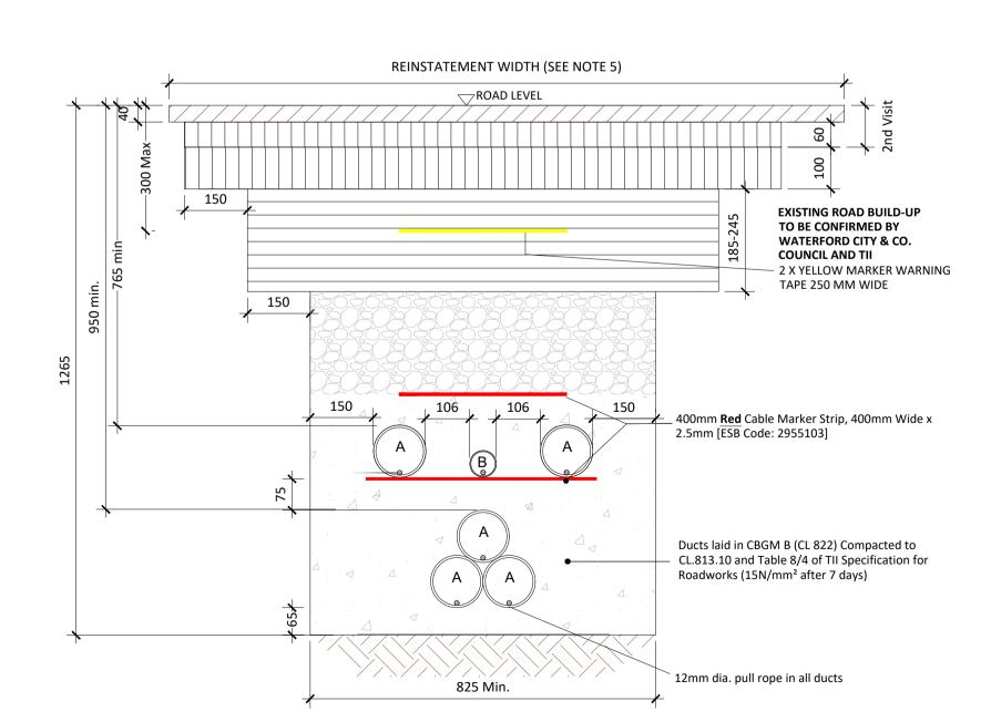
A = 125mm: Outer Diameter HDPE Duct, SDR=17.6 (Power) B = 63mm: Outer Diameter HDPE Duct, SDR=17.6 (Comms)
